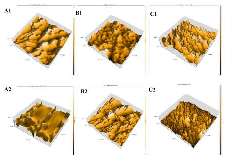
**Figure 4.** AFM images for manganese -cobalt -nickel oxide for the anode (A1, B1 and C1), and cathode (A2, B2, and C2) at different concentrations (0.05, 0.1, and 0.15 M) with constant molar ratio (1:1:1) at CD of 25 mA/cm<sup>2</sup> and 2 h of electrolysis
