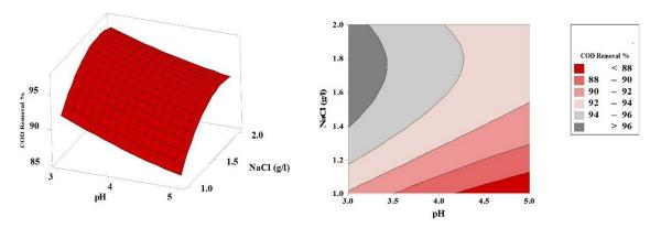
Figure 7. The impact of NaCl concentration and pH on COD elimination % at current density 60 mA/cm<sup>2</sup>, (a) 3D surface plot, and (b) Contour plot
