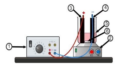
**Figure 1**. Electrodeposition cell schematic diagram: 1 – hot plate magnetic stirrer, 2) electrodeposition bath, 3 – cathode electrode, 4 – anode electrode, 5 – DC power supply
