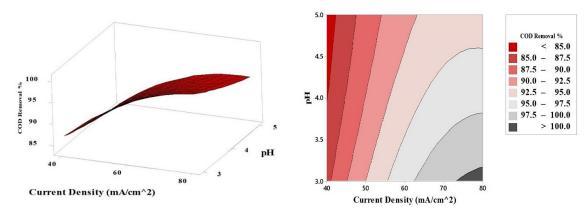
**Figure 6.** The impact of pH and current density on COD elimination % at NaCl concentration = 1.5 g/l, (a) 3D surface plot, and (b) contour plo
