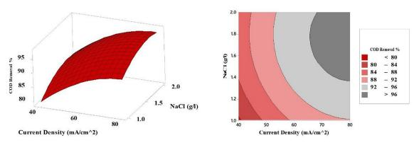
**Figure 5.** The impact of current density and NaCl concentration on COD removal % at pH = 4, (a) 3D surface plot, and (b) contour plot
